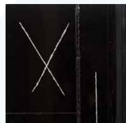
Aluminium | Epoxy + Top Coat | 1008 hr ASST
