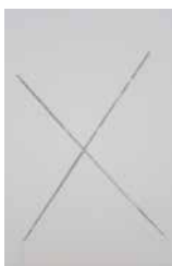
Aluminium | 1 layer powder coating | 1008 hr ASST
