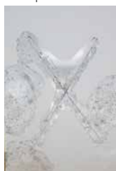
Aluminium | 1 layer powder coating | 1008 hr ASST
