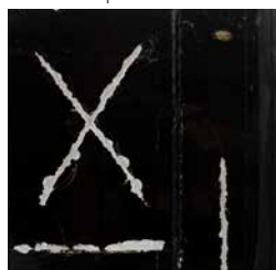
Aluminium | Epoxy + Top Coat | 1008 hr ASST
