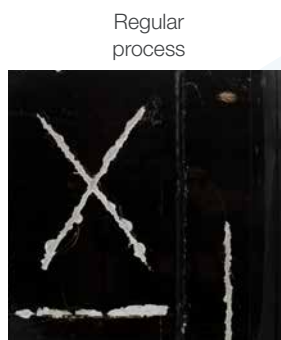
Aluminium | Epoxy + top coat | 1008 h ASST
