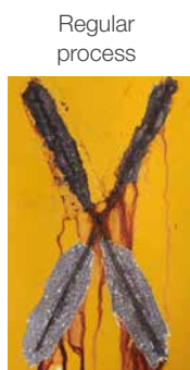
Steel | 1-layer powdercoat | 1008 h NSST
